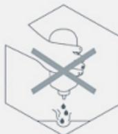
For normal cleaning of the frame surface use a solution of mild dishwashing liquid. Do not use scouring agent, paint thinner or . For stubborn dirt always use special cleaning agents that can be obtained from the window supplier or from a window specialist.
