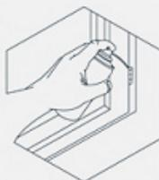
Lubricate the fittings at least once a year to ensure ease of movement at all times.
