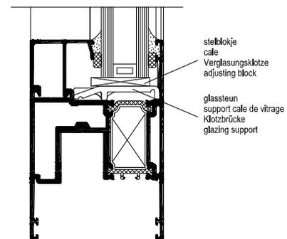
The following sketches indicate the different glazing blocks in different types of sliding elements.
