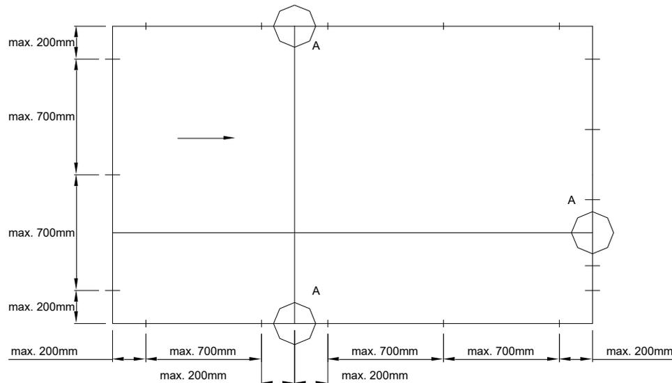
At least two fixings should be applied on all sides; the maximum distance to the corner is at least 200 mm.
