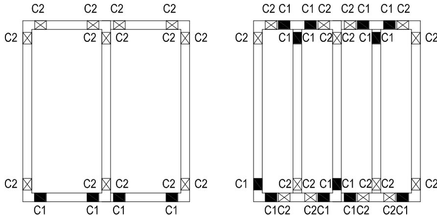
The glass weight of sliding panels should be distributed equally onto the rollers. The support blocks (C1) should consequently be fitted below at the height of the rollers.
